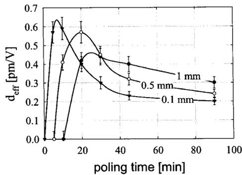
FIG. 2. Experimental values for the nonlinear coefficient ( $d_{33}$ ) against poling time for samples of different thicknesses ( $S$ ):  $S=1$  mm, full circles;  $S=0.5$  mm, open circles;  $S=0.1$  mm, full triangles. The lines are only a guide for the eye.
