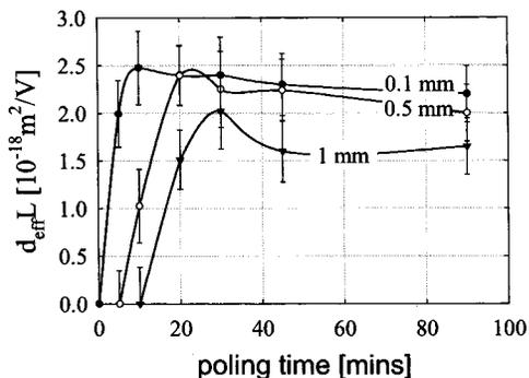
FIG. 4. Product  $d_{33}L$  of the measured nonlinear coefficient and thickness against poling time for three sample thicknesses:  $S=0.1$  mm, full circles;  $S=0.5$  mm, open circles;  $S=1$  mm, full triangles. The lines are only a guide for the eye.
