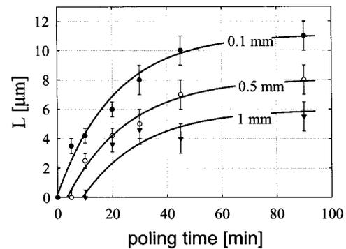
FIG. 3. Experimental values for the nonlinear thickness ( $L$ ) against poling time for samples of different thicknesses ( $S$ ):  $S=0.1$  mm, full circles;  $S=0.5$  mm, open circles;  $S=1$  mm, full triangles. The lines are the best-stretched-exponential fits for the experimental data.
