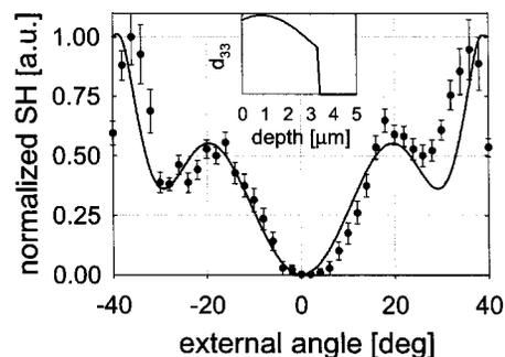
FIG. 1. Example of the noncollinear Makers fringe measurement on a 0.5-mm-thick HeraSil 1 sample thermally poled at  $280^\circ\text{C}$ , 4 kV, 10 min. Circles, experimental data; solid line, best fit obtained using  $L=3.4\ \mu\text{m}$ .
