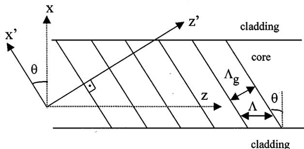
Fig. 7. Schematic of the tilted phase grating.
