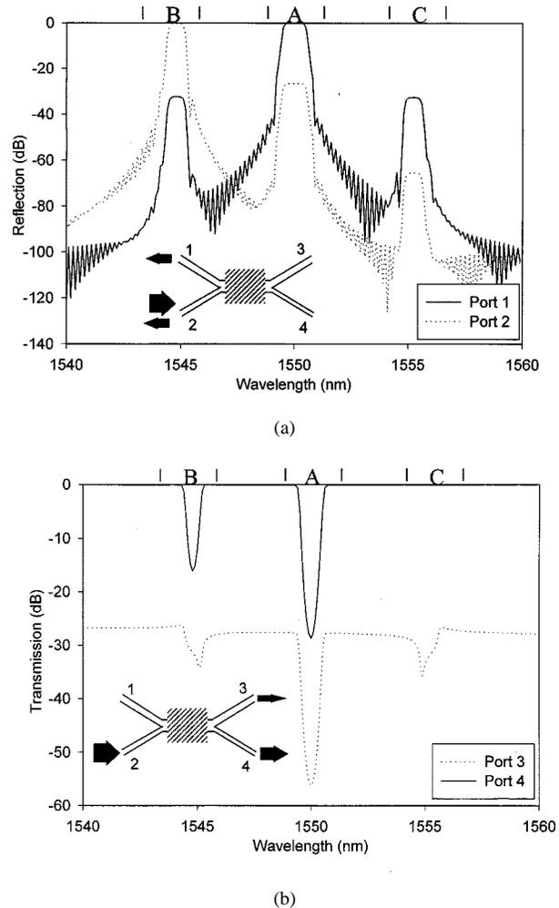
Fig. 11. Spectral response of the OADM with linear coupler and grating with nonoptimum tilt angle (Drop action): (a) reflection spectra and (b) transmission spectra.
