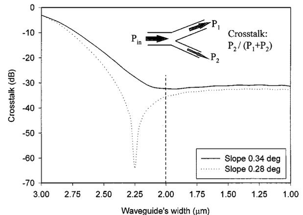
Fig. 4. Effect of the waveguide asymmetry to the crosstalk for two different slopes.
