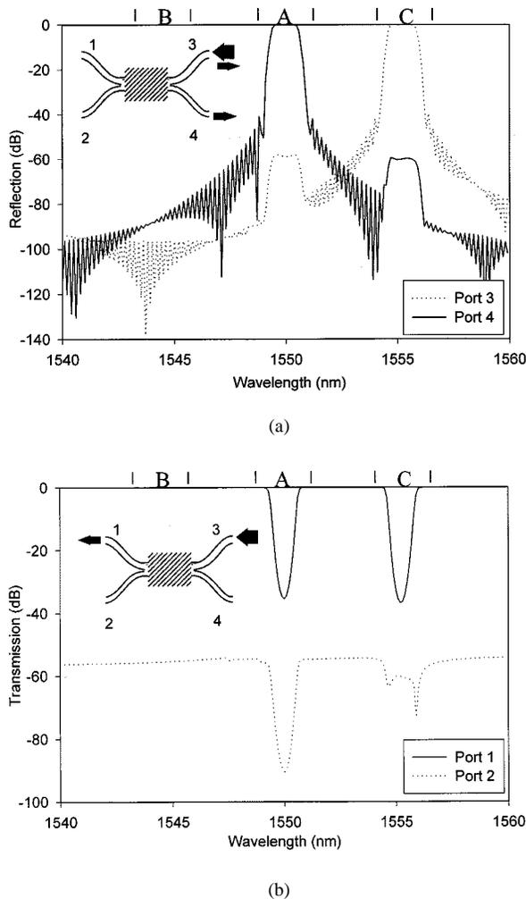
Fig. 14. Spectral response of the OADM with optimized null coupler and optimum tilt angle (Add action): (a) reflection spectra and (b) transmission spectra.
