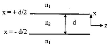
Fig. 15. Schematic of a three-layer symmetric waveguide.
