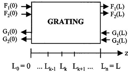
Fig. 6. Model for the calculation of the grating response.
