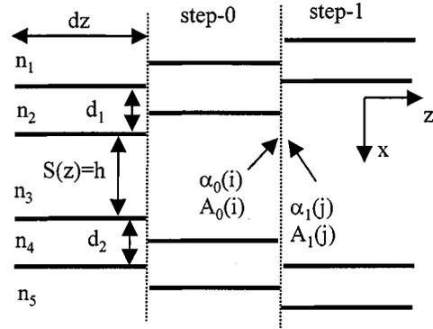
Fig. 2. Schematic of the step transition model.
