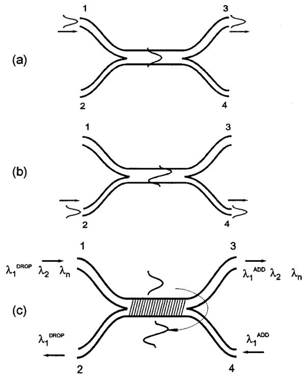
Fig. 1. Schematic of the OADM based on grating-assisted mode conversion in a null coupler. (a) Propagation of the even mode along the coupler. (b) Propagation of the odd mode along the coupler. (c) Cross-coupling of the two waist eigenmodes and demonstration of the OADM operation.
