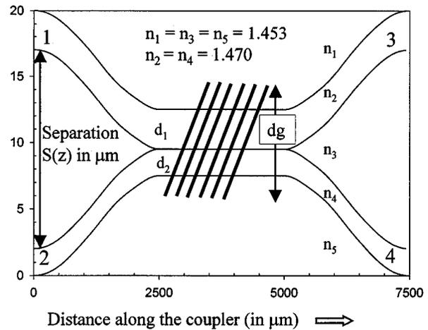
Fig. 3. Schematic and parameters of the tilted grating-assisted null coupler.
