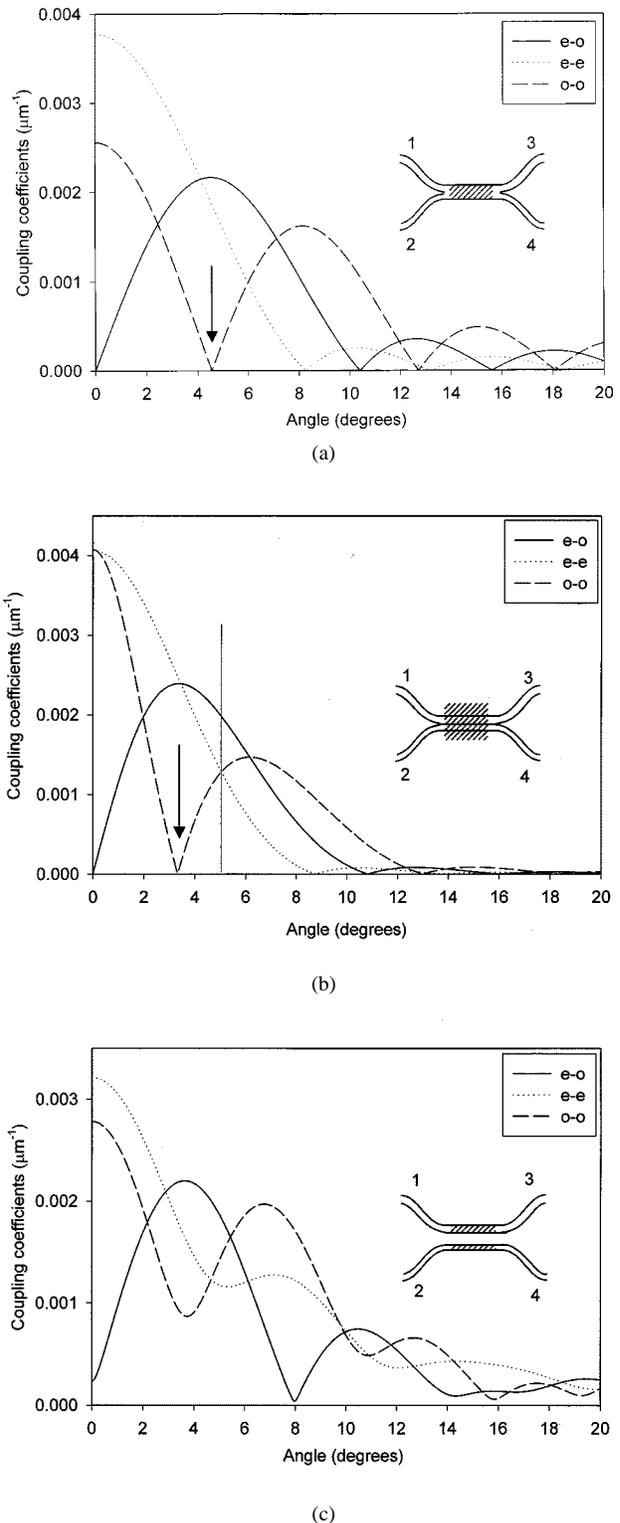
Fig. 8. (a) Coupling coefficients versus tilt angle when the grating is inscribed only at the single-core waist (waveguide's separation:  $h = 0 \mu\text{m}$ ). (b) Coupling coefficients versus tilt angle when the grating is extended deeply into the equally photosensitive cladding region. (c) Coupling coefficients versus tilt angle when the asymmetric waveguides at the waist of the coupler are separated by a distance:  $h = 1 \mu\text{m}$ .
