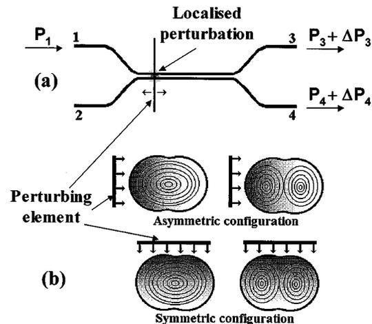
Fig. 1. (a) Principle of operation of the coupler characterization technique. (b) Schematic of the coupler-waist perturbation using an asymmetric (top) or symmetric (bottom) configuration.
