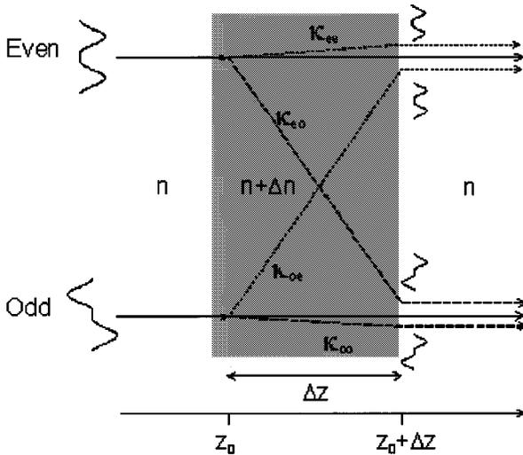
Fig. 2. Schematic of even and odd eigenmode self-coupling ( $\kappa_{ee}$ ,  $\kappa_{oo}$ ) and crosscoupling ( $\kappa_{eo}$ ,  $\kappa_{oe}$ ) induced by the external perturbation  $\Delta n$ , represented by the shaded area.
