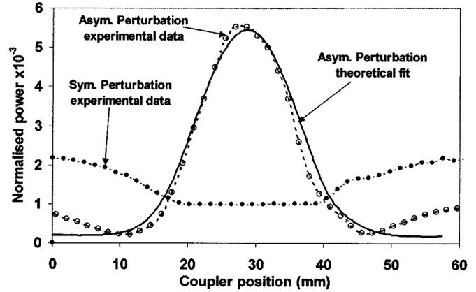
Fig. 3. Characterization of a half-cycle coupler using a local perturbation in both an asymmetric and symmetric configuration. The asymmetric perturbation was fitted using the symmetric perturbation data.
