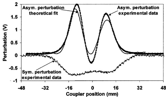
Fig. 4. Characterization of a full-cycle coupler using a local perturbation in both an asymmetric and symmetric configuration. The asymmetric perturbation was fitted using the symmetric perturbation data.
