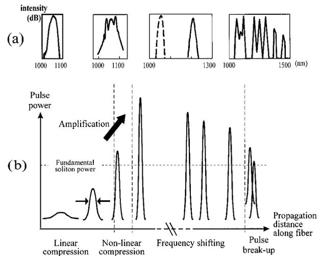
Fig. 2. Representation of the pulse evolution with propagation distance along the holey fiber amplifier: (a) frequency domain, optical spectra; (b) time domain, pulse duration/peak power.
