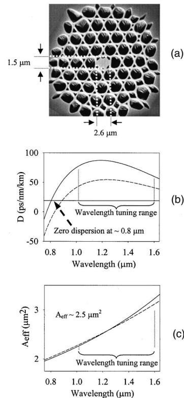
Fig. 5. Characteristics of the  $\text{Yb}^{3+}$ -doped holey fiber. (a) SEM of the structure, showing the dimensions of the elliptical core. (The metallic coating required for producing SEM images enlarges the fine silica bridges by  $\sim 50 \text{ nm}$ , which is taken into account when we calculate the fiber characteristics.) (b) Dispersion predictions for the two principal polarization axes. (c) Effective mode area ( $A_{\text{eff}}$ ) predictions for the two principal polarization axes.
