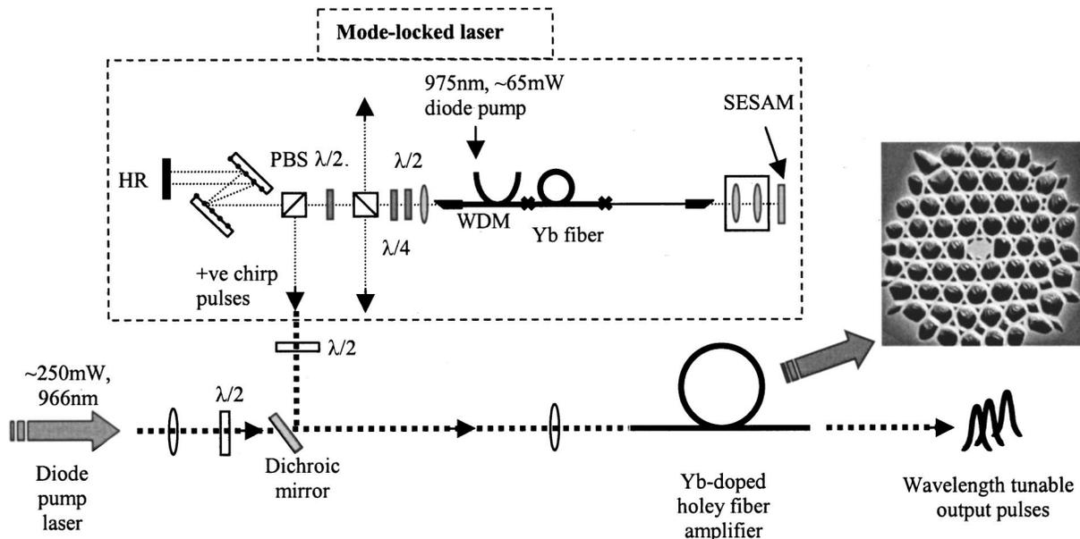
Fig. 1. Experimental setup, showing the in-house mode-locked  $\text{Yb}^{3+}$  fiber seed laser (diode pumped), the launch arrangement for seeding the pulses and the pump laser to the  $\text{Yb}^{3+}$  doped holey fiber amplifier, and an inset SEM of the holey fiber structure. HR, high-reflectivity mirror; +ve, positive, WDM, wavelength-division multiplexer; PBS, polarizing beam splitter.
