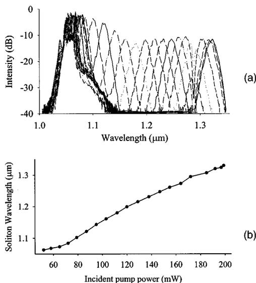
Fig. 6. Tunable single-color solitons: (a) superimposed spectra of the solitons shifted to progressively longer wavelengths (1.06–1.33  $\mu\text{m}$ ), (b) plot of the soliton wavelength versus amplifier (incident) pump power.
