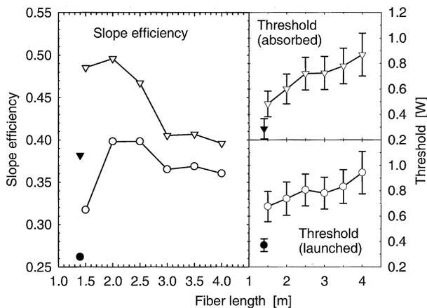
Fig. 6. Slope efficiency and pump threshold power versus fiber length, with respect to launched pump power (circles) and absorbed pump power (triangles). Empty symbols: single-ended pumping at 915 nm (fiber lengths 1.5–4 m). Filled symbols: single-ended pumping at 980 nm (single fiber length of 1.4 m).
