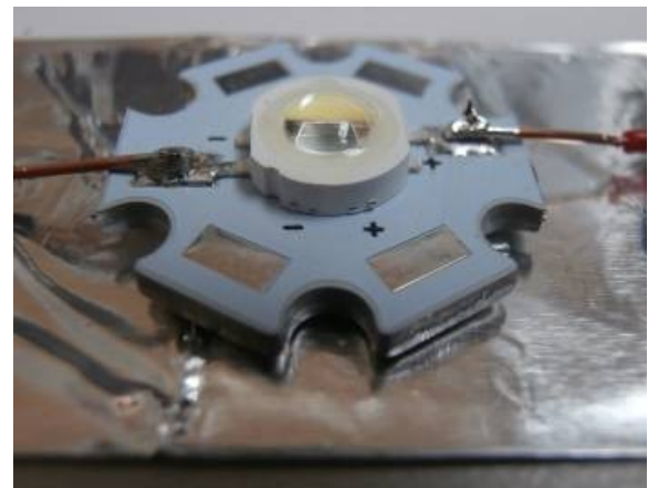
Fig. 187 Images showing wires soldering for the realization of the LED source.
