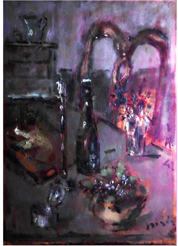
Fig 62 Total of the painting in ultraviolet fluorescence. Differentiation of pictorial materials. Stronger UV fluorescence of white pigments.
