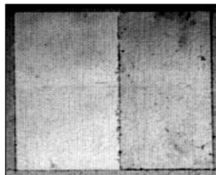
Fig. 176b Image (530 nm) of a frame where difference between varnished and not varnished part is visible.
