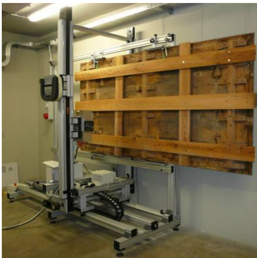
Fig. 91 The painting during the acquisition of radiographic images with the 2D radiographic scanner.
