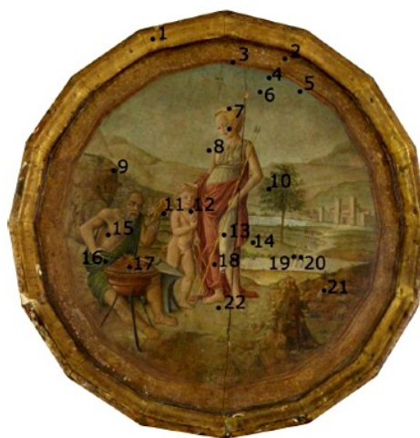
Fig. 139 Measuring points analyzed by XRF (I recognition).
