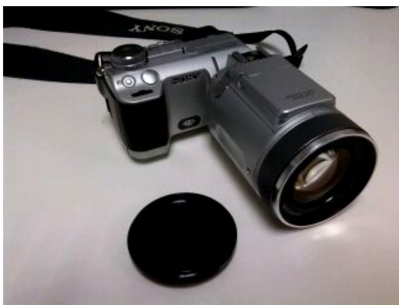
Fig. 215 Sony photo camera (Cyber Shot F717) with Si CCD for IR reflectography and the IR filter (F.2 - 950 nm).
