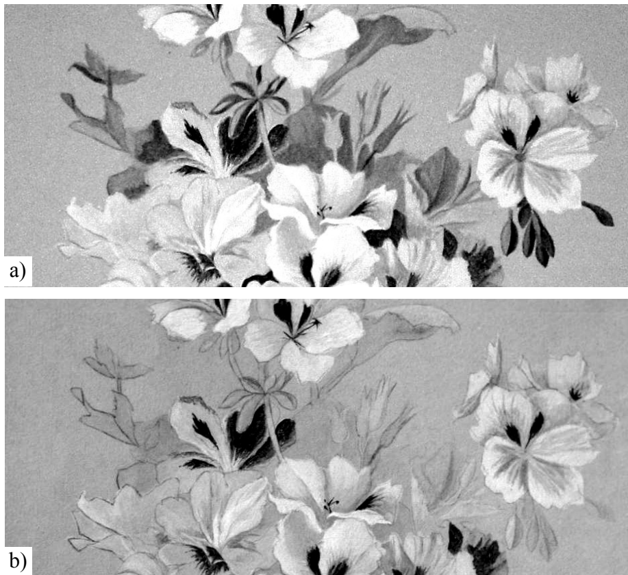
Fig. 217a-b Comparison of a detail. a) IR Reflectography acquired by Si CCD; b) IR Reflectography acquired by InGaAs detector (Peccenini, 2012).
