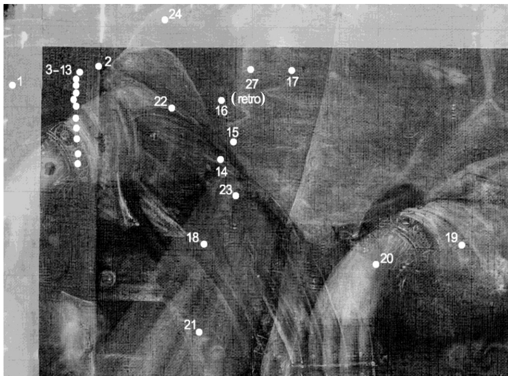
Fig. 126 Measuring points analyzed by XRF, indicated on the radiography.
