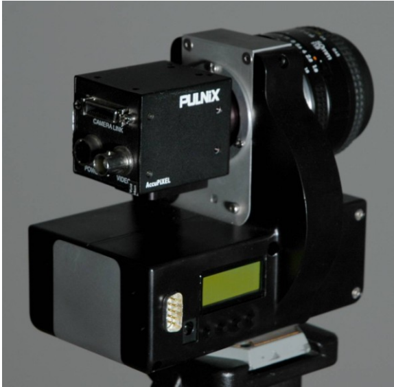
Fig. 205a Image spectroscopy device, equipped with Pulnix TM-1325 camera
