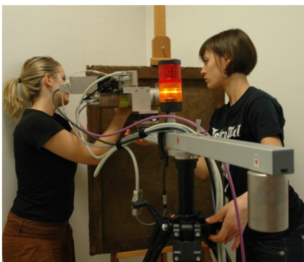
Fig. 209 The XRF device. Positioning of the instrument on a painting, on different areas to be investigated.
