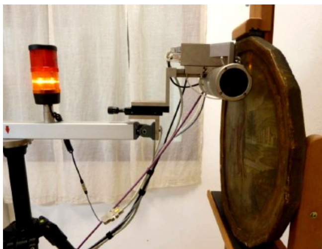
Fig. 138 The desco , while performing XRF analysis.
