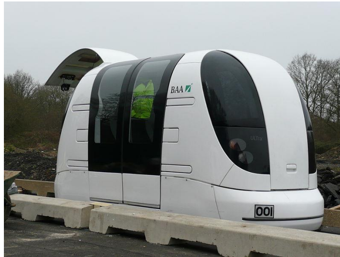
Figure 3.2 ULTra PRT vehicle on a test track
