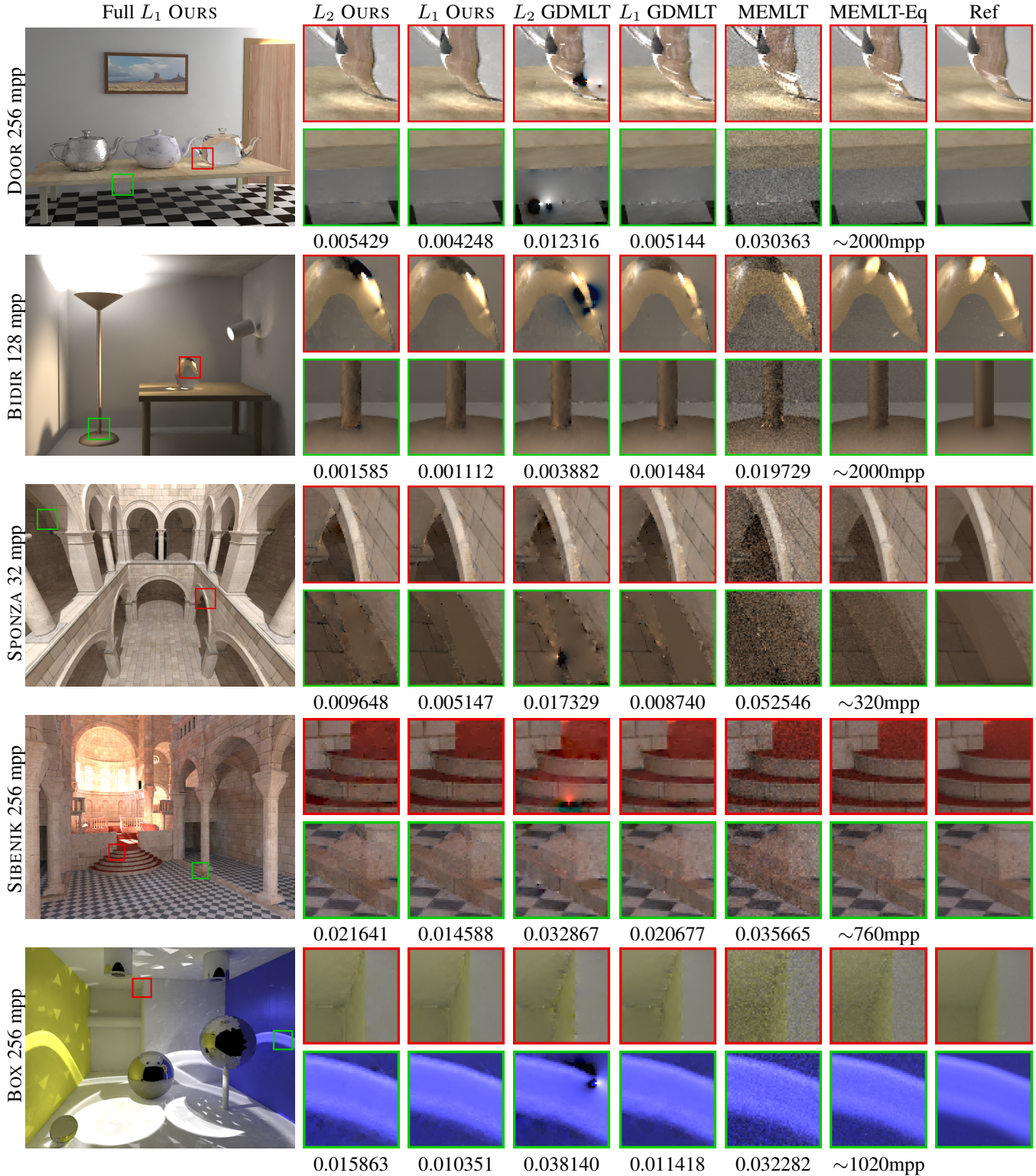
Figure 13: Our proposed method using L_2 and L_1 reconstruction compared to gradient-domain MLT and manifold exploration MLT using approximately the same number of mutations per pixel (mpp). MEMLT-Eq shows MEMLT with more samples in order to achieve approximately the same quality in terms of rMSE as L_1 OURS. The numbers below the close-ups with exception of MEMLT-Eq show the rMSE of the full images. All references were generated using MLT with 32k mpp.
