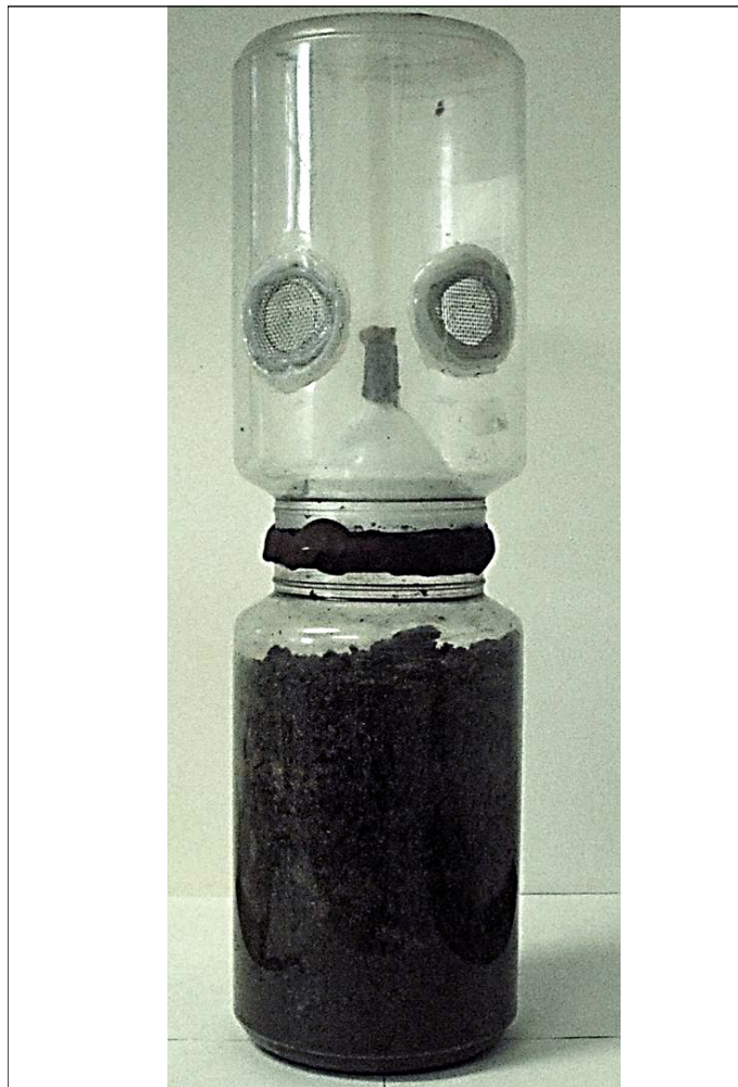
Fig. 8. Small hive beetle pupation chamber with an adult beetle funnel trap fitted on top. There is an inverted funnel in the middle that beetles from the pupation chamber (container with soil) crawl through to access the adult chamber (top). The adults can be fed with honey water that is sprayed through the ventilation holes in the upper container.
