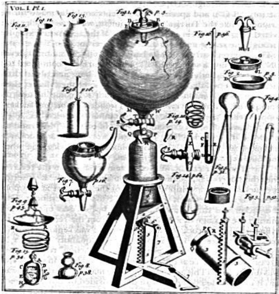
Fig. 2. Boyle's air pump was an advance over Von Guericke's spheres in that it provided a glass receptacle into which candles, mice, and other objects could be placed for experimentation. Air was ratcheted out from a cylinder and piston attached through a stopcock to the receptacle. After each cylinder of air was evacuated, the stopcock was closed and the ratchet and piston reset.
