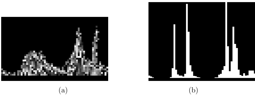
Figure 5.6: (a) Hue-Saturation histogram for the image toypark.png , the saturation values correspond to the vertical axis and the hue values correspond to the horizontal axis. The selected parameters are 18 and 6. The level grey represents the number of occurrences, from black for 0 occurrences to white to the maximum number of occurrences. (b) Hue histogram for the same image, the horizontal axis represents the hue values and the vertical one the occurrence values. The selected parameters are the same as before.
