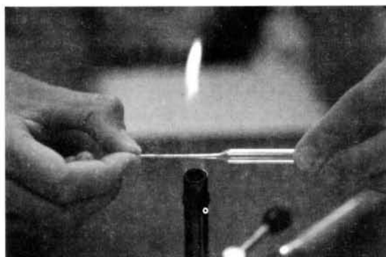
Fig. 5. Pulling a Pasteur pipette: the thin part is rolled back and forth over the flame of a bunsen burner. When the glass is soft, the pipette is moved away from the flame and quickly pulled.
