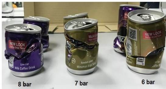
Figure 5. The desired size of Nescafe brand of the cans according to the pressure supply
