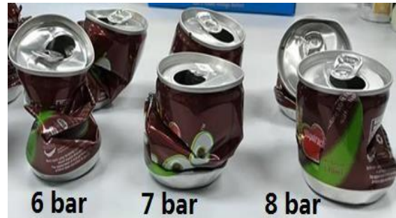
Figure 8. The desired size of Oligo brand of the cans according to the pressure supply
