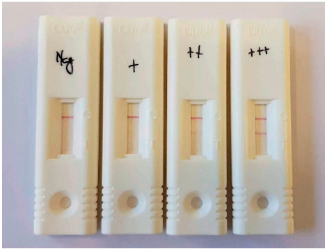
Figure 1: Lateral flow devices, showing from left to right a negative result, followed by increasing test line intensity. The control line is visible at the top, while the test line appears below the control line.
