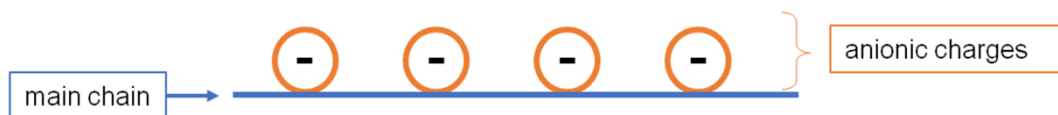
Figure 5. Schematic representation of the basic structure of a polycondensate superplasticizer; modified from [5].
