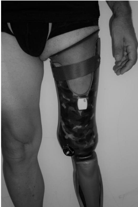
Figure 5: 3D-acceleration sensor fixed centrally on the front side of the prosthetic socket
