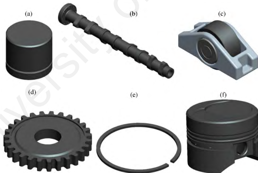
Figure 2.5: Automotive applications of DLC coatings: (a) tappet, (b) camshaft, (c) finger roller follower, (d) camshaft sprocket, (e) piston ring, and (f) piston
