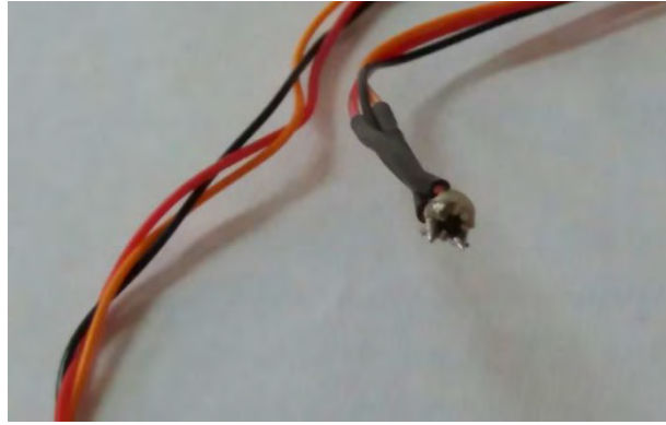
Figure 3.11: Giant magnetoresistance (GMR) magnetometer chip mounted on Printed Circuit Board (PCB)
