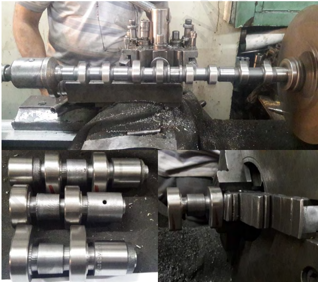
Figure 3.8: Cutting of original camshaft to take out camlobes using lathe machine
