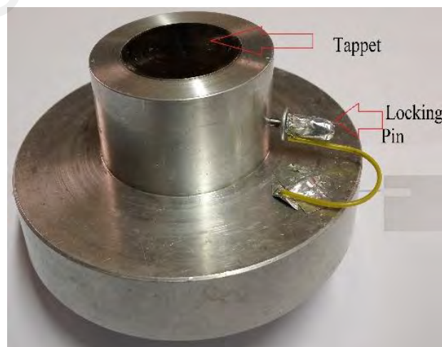
Figure 3.17: A specially-designed jig for holding the tappet during surface profilometry
