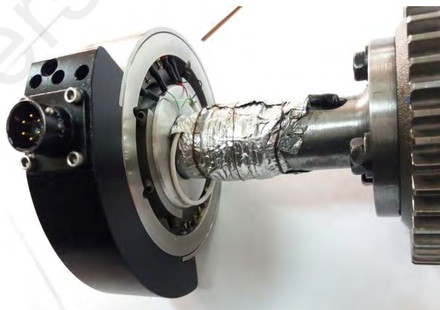
Figure 3.14: Michigan Scientific B6-2 slip ring assembly
