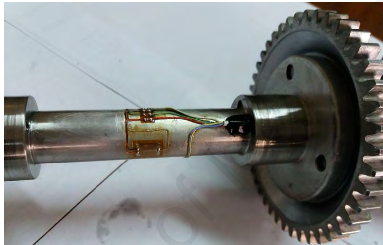
Figure 3.13: Strain-gauge-based torque tube integrated with camshaft
