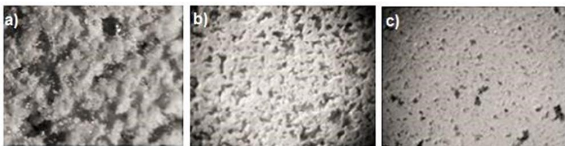
Figure 5. Microstructure of the surface of shell molds ( \times 60 ): a) Armosil, b) Ludex c) ethylsilicate
