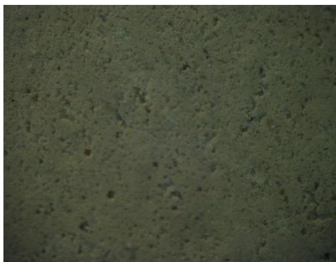
Figure 6. Contact surface of a ceramic mold based on a Chinese binder GN-25 (25% \text{SiO}_2 content) + 10% latex and quartz sand ( \times 60 )
