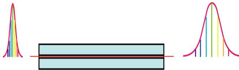
Figure 3.3: Dispersion effect in an optical fibre [71]
