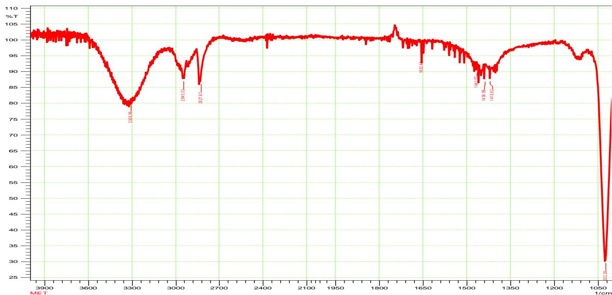
Figure 1-8. IR spectrum of methanol.
