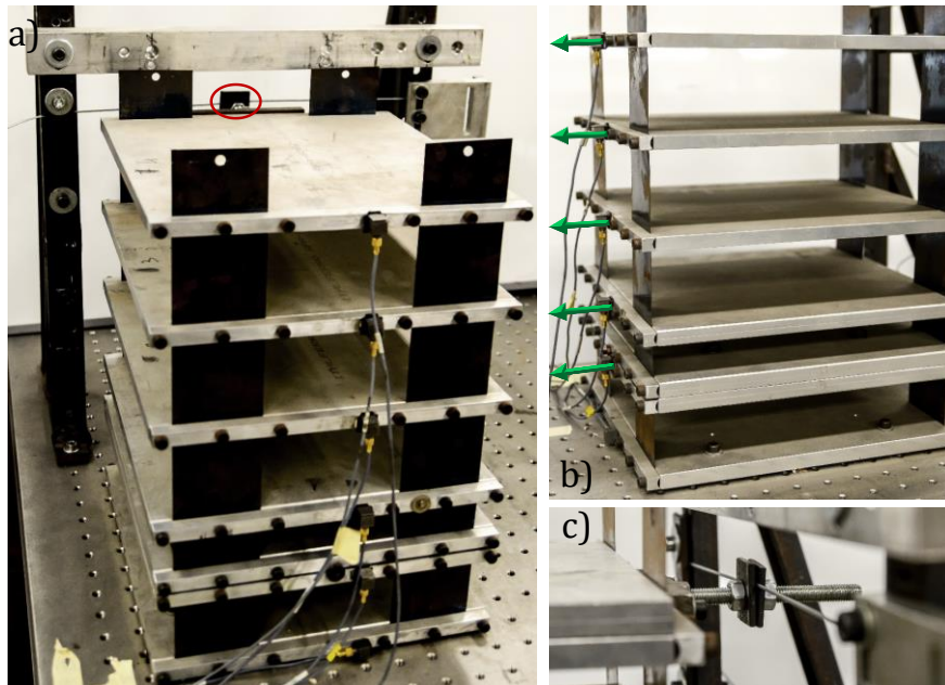
Figure 4.9: Photos of the experimental setup. a) Overall view with nonlinear link highlighted in red; b) Overall view with motion directions in green; c) Particular of the nonlinear link (thin wire).
