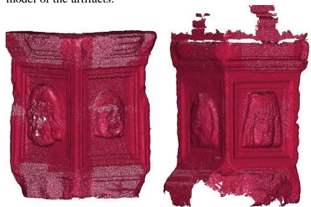
Figure 9 The final points clouds of the four theatrical masks obtained with the HandyScan 3D
