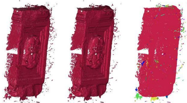
Figure 8 Raw data with outliers (left), the point clouds after the noise reduction (centre), the founded outliers (various color in the image) using the distance filter (right)
