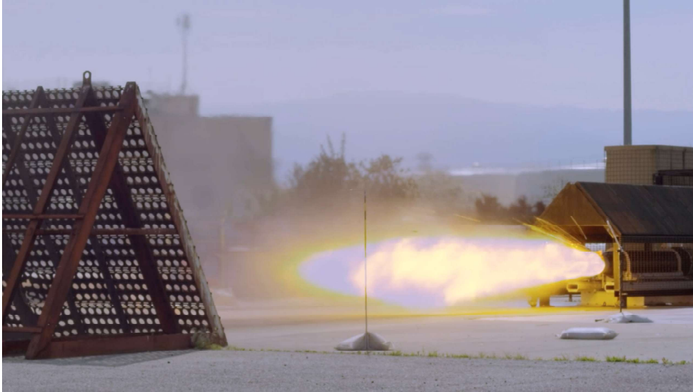
Figure 2.3: Peregrine static test. Credits: NASA Ames Research Center.
