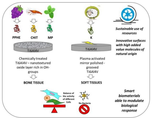
Results and discussions: Un-treated Ti6Al4V surface has not functional groups suitable for chemical grafting. In order to improve functionalization ability, a nanotextured oxide layer rich in OH-groups has been obtained by a chemical treatment [1] and natural biomolecules grafted with high chemical stability for an increased biological response of bone tissue (Ti64-F-PPHE: increased mineralization, redox and radical scavenging activity) or antibacterial action (Ti64-F-MP).
