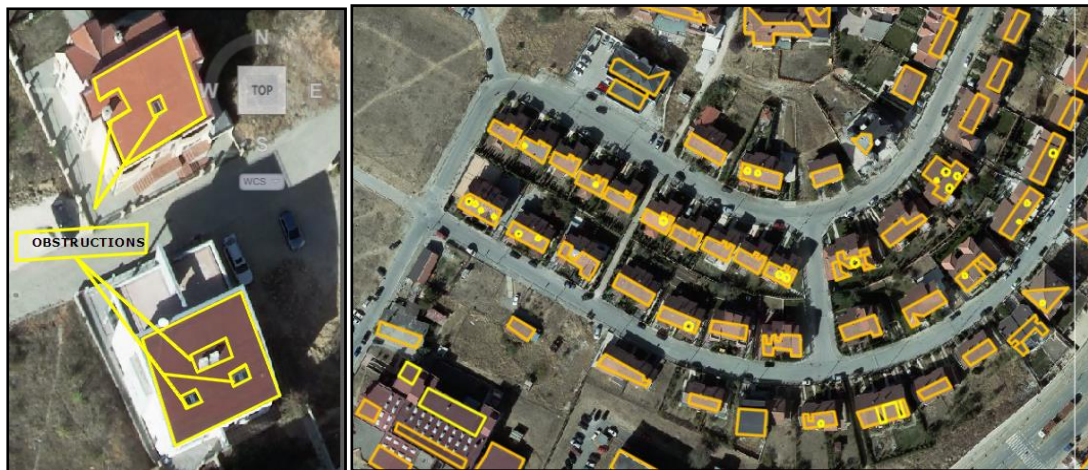
Figure 3. The roof surface which is appropriate for installing solar collectors
