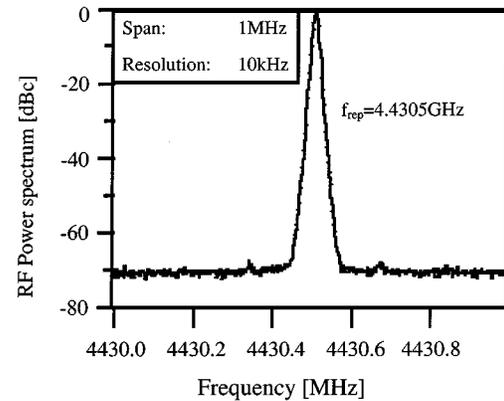
Fig. 2. Radio-frequency spectrum of the VECSEL power output showing mode locking without  $Q$ -switching instabilities at a repetition rate of 4.43 GHz. The signal was obtained with a 50-GHz photodiode and a 26-GHz amplifier and spectrum analyzer.
