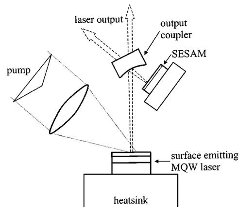
Fig. 1. Mode-locked diode-pumped VECSEL cavity with SESAM.
