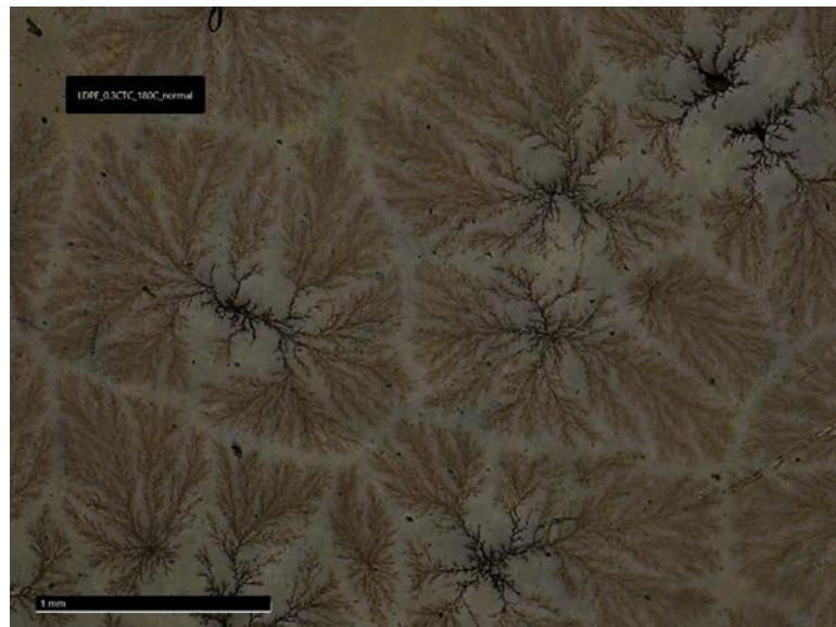
Figure A.18: LDPE_0.3CTC_180C_normal areas with unusually high CTC branch density.
