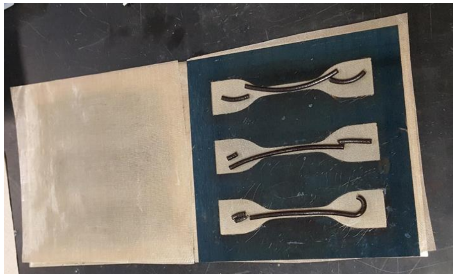
Figure 2.4: Mold for tensile bars between Teflon™ coated fiberglass sheets for ease of removal.
