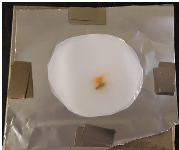
Figure 2.1: Image showing TTF (orange) and TCNQ (greenish-brown) powders between two LDPE films prior to compression-molding.
