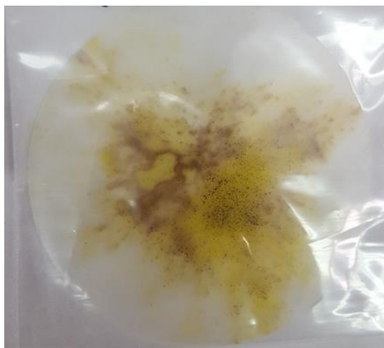
Figure 2.2: Image showing the film after the initial press, the TTF and TCNQ are embedded in the LDPE matrix.
