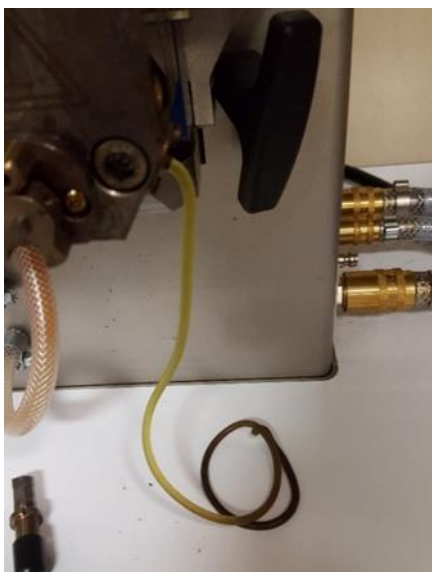
Figure 2.3: Image showing transparent yellow composite extrudate cooling into a dark black/ brown color at room temperature.
