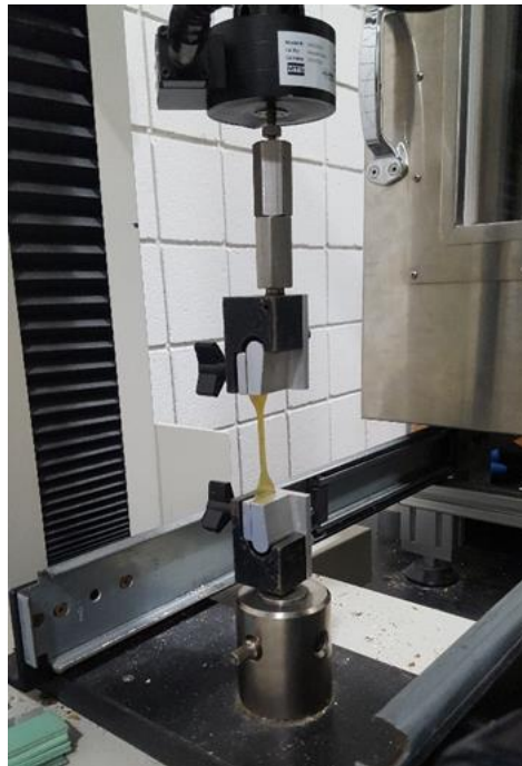
Figure 2.14: Representative tensile testing setup of LDPE_0.16CTC_180C_normal with DIN EN ISO 527-1 molded dog-bones.
