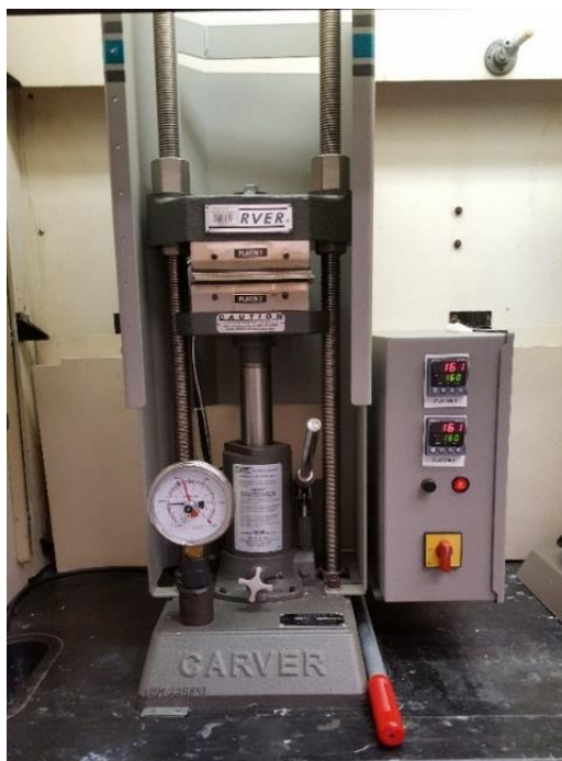
Figure 2.7: Slow cooled samples left on the Carver™ Melt-press as it cools to room temperature.
