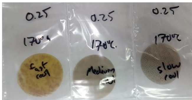
Figure 2.8: Images showing the composite samples at the various cooling rates.
