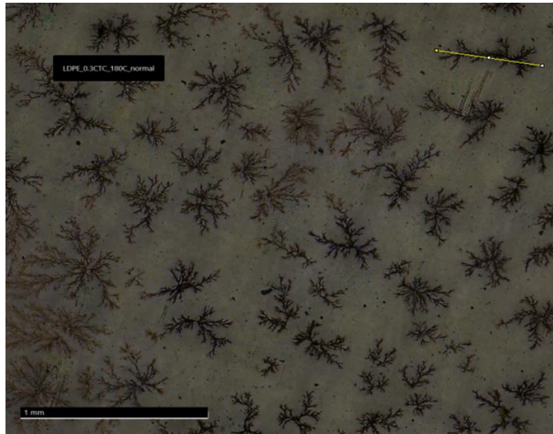
Figure 2.10: Representative image of longest diameter measurement of a dendritic CTC particle in LDPE_0.3CTC_180C_normal.
