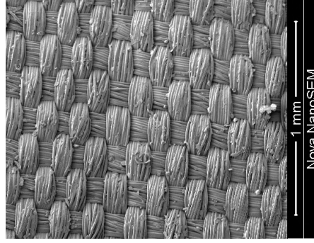
Figure 3.12 Visualization of the microscopic structure of a woven PET graft of a Medtronic Endurant™ II SG using scanning electron microscope.
