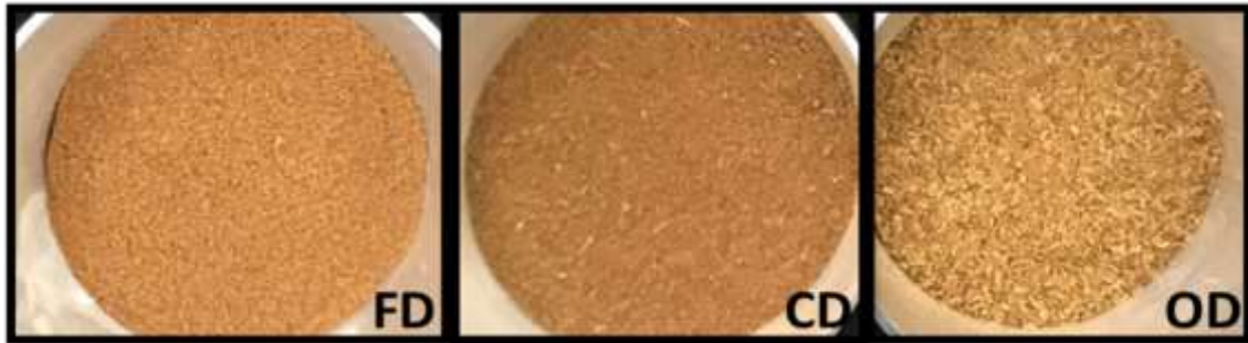
Figure 1. Coffee pulp/husk flour obtained by freeze drying (FD), convective drying after wet process (CD), convective drying after dry process (OD).
