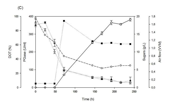
Fig. 2. Cultivation profile of *A. sojae* growing on orange peel and apricot pomace in 1-L bioreactors operated at (A) constant airflow and agitation speed (1 vvm, 600 rpm), (B) constant airflow (1 vvm) and cascading agitation speed, (C) constant agitation speed (600 rpm) and cascading airflow.
