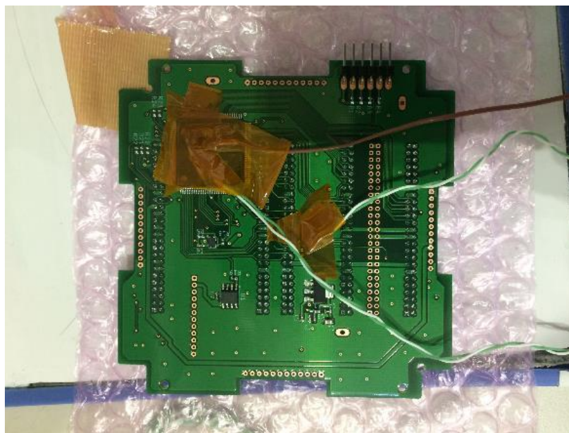
Figure 5-7. Thermocouples placed on the CPLD of SoftCIB
