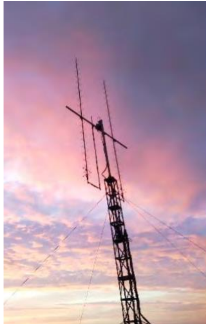
Figure 6-8. UHF antenna for BIRDS ground station at Kyutech. BIRDS-3 uses UHF band for uplink and downlink. Image source [66].
