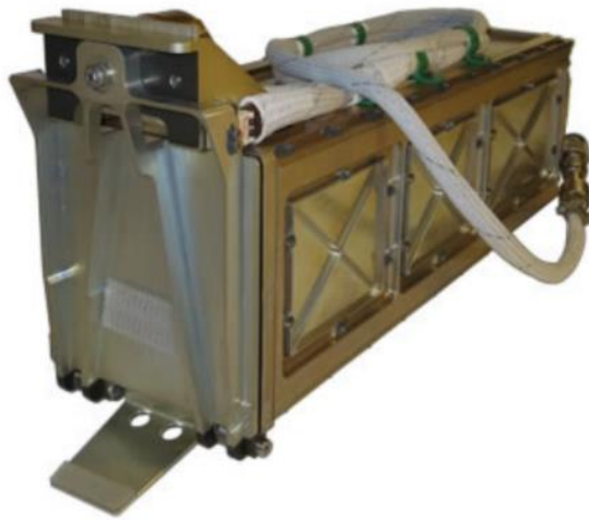
Figure 2-4. Poly Picosatellite Orbital Deployer (P-POD) developed by Cal Poly [23]
