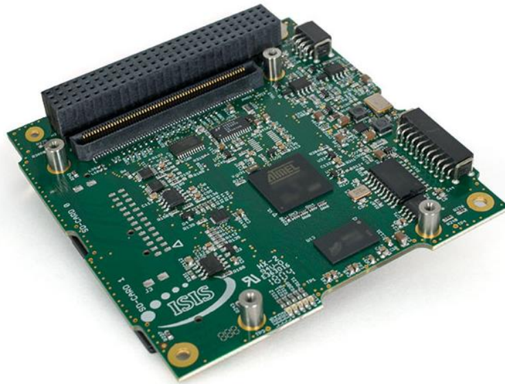
Figure 2-7. Onboard Computer board with PC104 interface, developed by ISIS.
