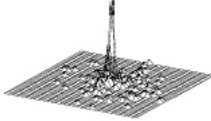
Figure 2.2: An example of a peak in the discrete cross correlated function.
