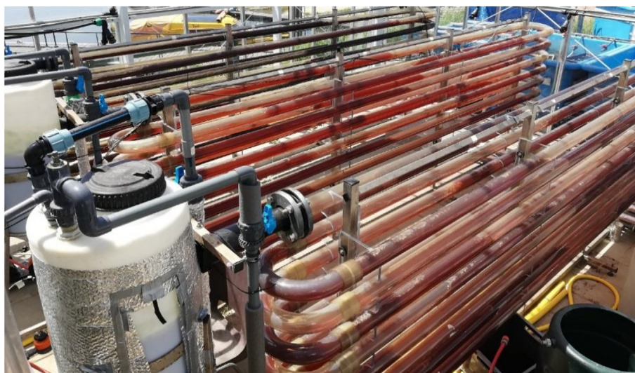
Fig. 1. Picture of three tubular photobioreactor operated with Rhodomonas sp. as seen from the North-East.
