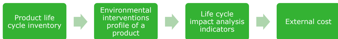
Figure 2 Steps from a description of all processes to an estimate of external costs
