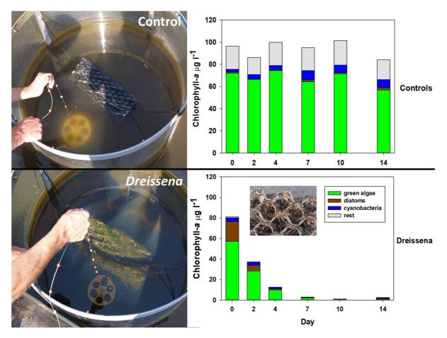
Fig. 5 Enclosure experiment with four enclosures that received an empty crate each and four that received a crate with dreissenids that cause strong reduction of the phytoplankton biomass (Waajen et al., 2016b; pictures G. Waajen)
