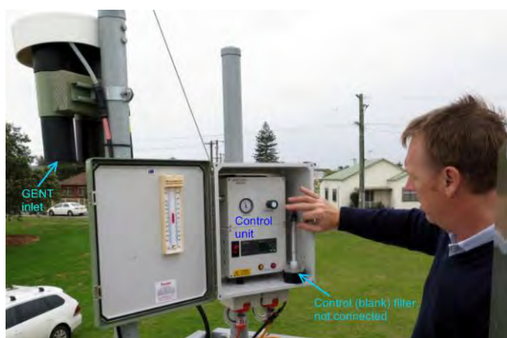
Figure 11 Details of the GENT sampler at the Stockton site being inspected by Peter Crabbe
