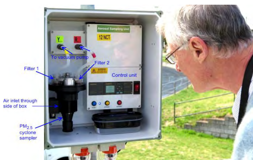
Figure 10 Details of the ASP Sampler at the Newcastle site being inspected by David Cohen
