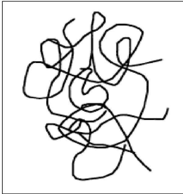
Figure 2.5 Molecular arrangements in amorphous polymers (Mazumdar, 2002)
