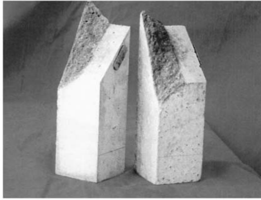
Figure 23: Brokenshire torsion test. Experimentally obtained crack surface. Adapted from [38].
