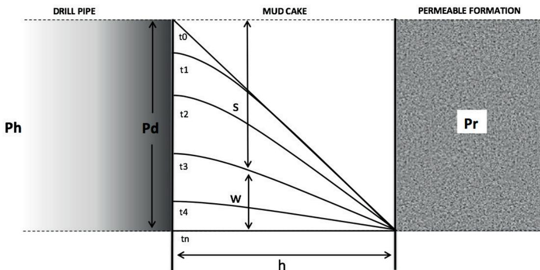
Outmans created *Equation 5*, that determines the half value time ( $T$ ), which is the sticking time required to let the friction force increase to 50 percent of its maximum value. If we correlate *Equation 5* with Darcy's Law expressed as *Equation 6* (considering the mud cake as a homogenous porous media), we obtain *Equation 7*:
