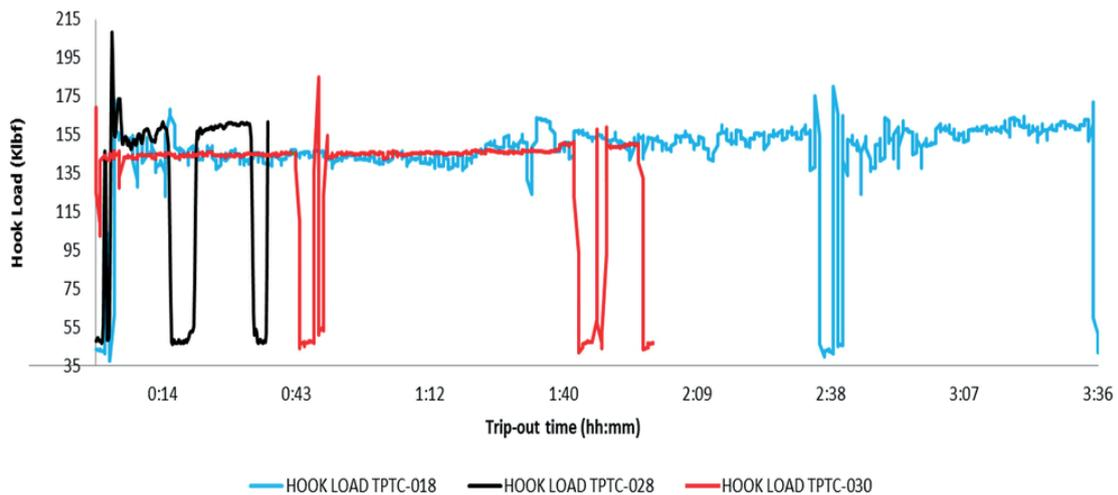
It is relevant to point out that wells TPTC-018 and TPTC-030 had a risk zone of similar height, and also TPTC-030 had a higher inclination, which implied that torque and drag on TPTC-030 should have been higher with the same drilling mud properties. However, the addition of diesel proved to be effective on dynamic conditions, since it brought a more stable behavior of trip-out parameters, reduced their magnitude and enabled a significant reduction on tripping time.
