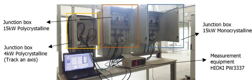
Figure. 2. Acquisition of data from the Microgrid HIOKI PW3337 - LabVIEW
