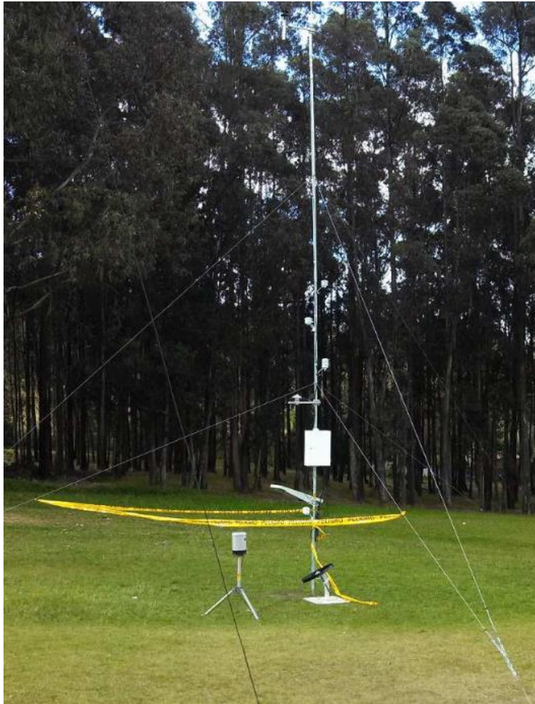
Figure 3. Portable meteorological station
