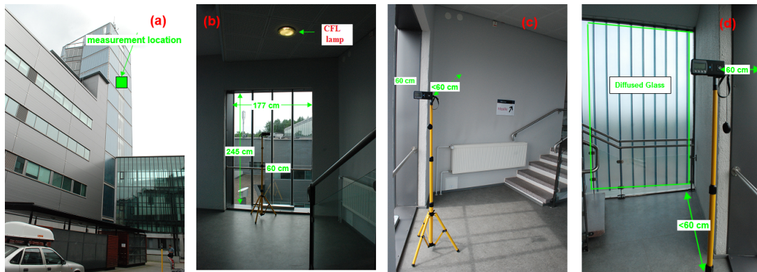
Figure 15: Open exterior daylight measurement location; (a) the measurement location is at the fifth floor in Network Oasis tower that is shadow free from nearby buildings (b) according to the position of the south facade window, the south and north horizontal measurement directions (c) the west cardinal horizontal measurement direction (d) the east cardinal horizontal measurement direction
