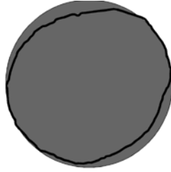
Figure 4.2: Study of the robustness w.r.t mismodeling the boundary shape. Measurement domain \Omega ( \partial\Omega is shown with solid line) and model domain \tilde{\Omega} shown as gray patch are used for experiment in Section 4.3.1.
