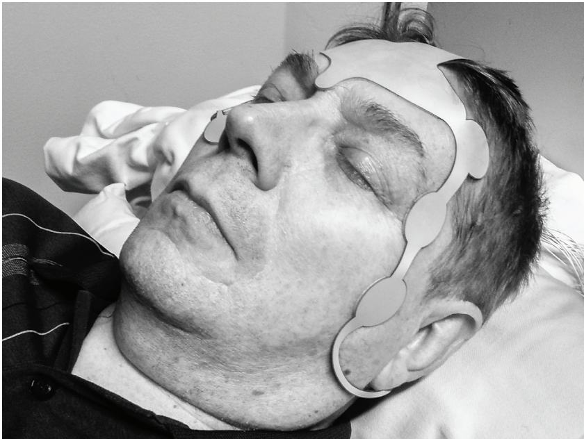
Figure 7.4. A silver-shielded EEG electrode set attached to a volunteer's head. The silver layer was printed on the front side of the polyester film to protect the electrode set from environmental electromagnetic artefacts. The use of this photograph has been permitted by the volunteer.
