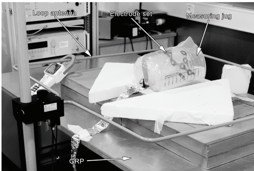
Figure 7.5. Measuring jug attached screen-printed EEG electrode set were placed 10 cm above the ground reference plane (GRP) inside a loop antenna in a pulsed immunity test system.
