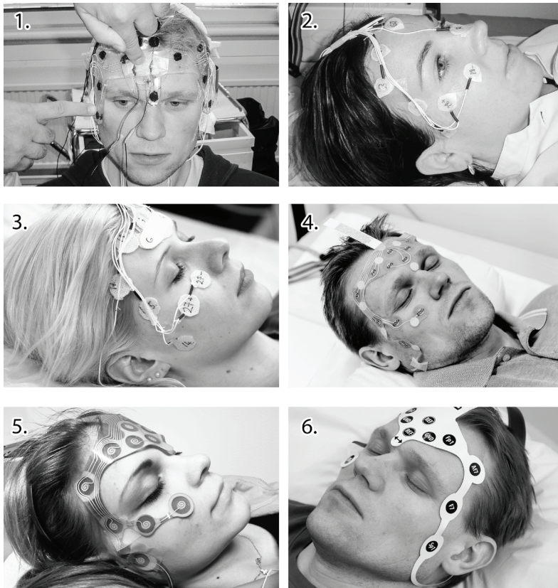
Figure 7.1. These images illustrate the evolution of the developed electrode set during the last four years. Prototype generations are presented in numerical order. Images 1-3 represent prototypes of handmade EEG electrode set and 4-6 show prototypes of the screen-printed EEG electrode set. The use of these photographs has been approved by the volunteers.
