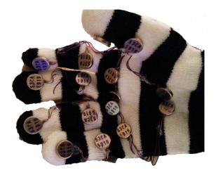
Figure 2. The underside of the Leap Motion Haptic Glove with 16 vibration motors
