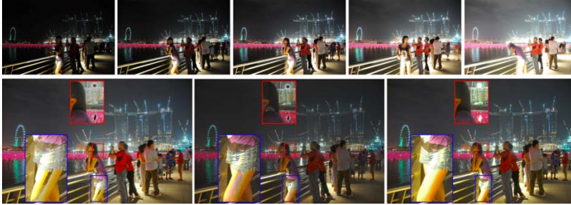
Fig. 3.10 De-ghosting visual comparison in a night scene with (top) input images, using (bottom-left) Photomatix, (bottom-middle) Photoshop and (bottom-right) [P5].
