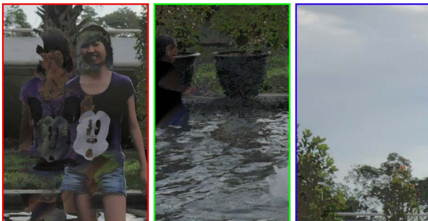
Fig. 6.2 HDR image synthesized using entropy-based de-ghosting algorithm proposed in [82]. Obvious ghosting artifacts are seen in red and green blocks. The implementation was downloaded from original author's website in the binary of PhotoSphere 1 . The processing time was around 5 seconds on a Mac Pro desktop. An HDR image was synthesized from the binary app, and it was then been compressed using Photomatix through tone mapping.
