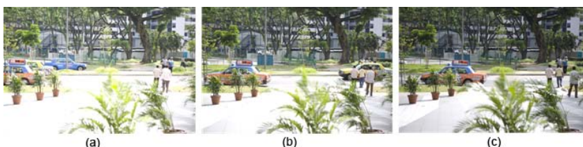
Fig. 5.1 Images captured with moving people and vehicle using different exposures settings: (a) +1 EV, (b) 0 EV, and (c) -1 EV. Although they are captured at the same scene within a short period of time, the similarity index (SSIM) between each pair of images appears to be low at SSIM(a,b)=0.6685 and SSIM(a,c)=0.4216 .
