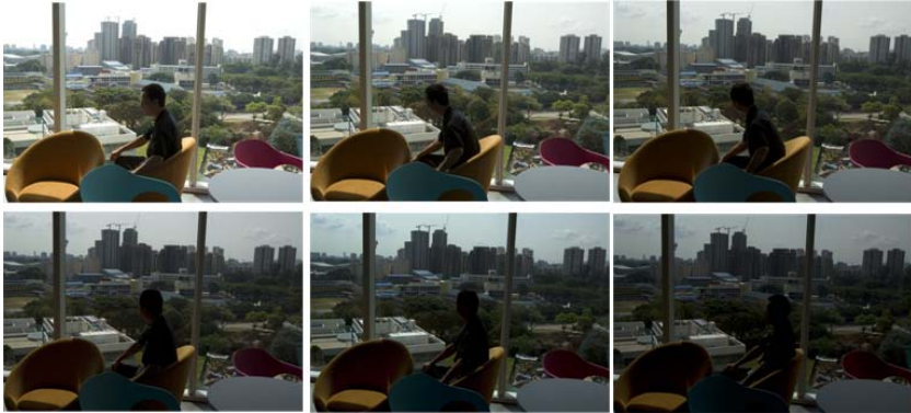
Fig. 5.2 Sequence of images contain camera movement, moving object, and exposure difference of EV interval of 2/3. Images are marked as 1 to 6 from left to right, top to bottom.
