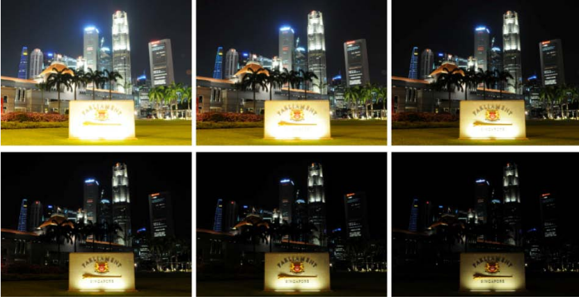
Fig. 2.1 A sequence of exposure bracketing images from the highest exposure (top left) to the lowest exposure (bottom right). The image of high exposure captured the detail of dark area with the saturation in the bright area, while the image of low exposure captured the bright area with the saturation in the dark area.
