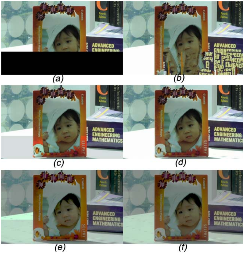
Fig. 2.5 Patching results of a degraded image from an exposure bracketing set shown in Fig. 2.2. (a) Original degraded image, (b) fixed image using exemplar-based inpainting [54], (c) fixed image using CRF [58], (d) fixed image using the proposed method, (e) HDR image synthesized with degraded image, and (f) HDR image synthesized with patched image [P1].
