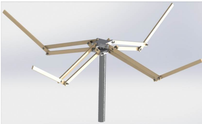
Figure 6. Compact and deployed forms of the solid model with single four-bar loop per limb
