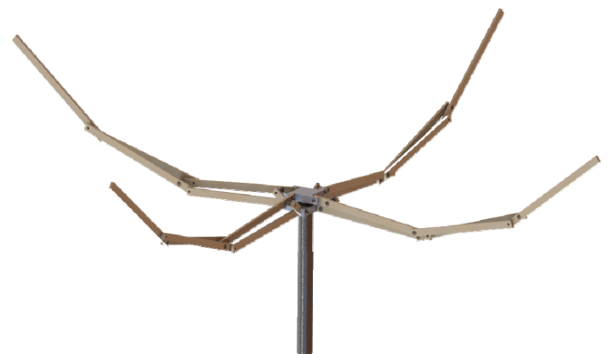
Figure 13. The model with two four-bar loops per limb and limbs bent upwards
