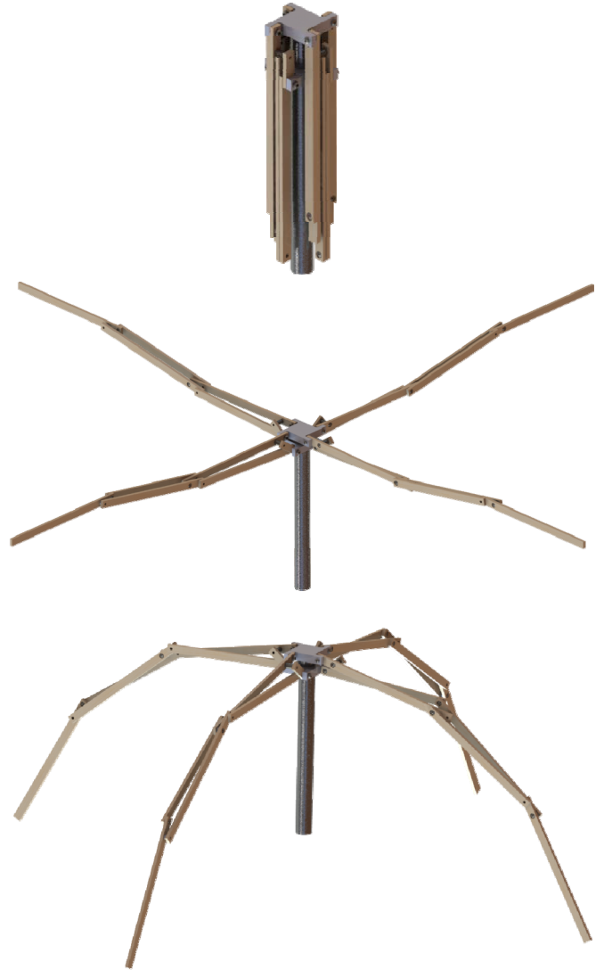
Figure 12. Compact, fully-open and fully closed forms form of the model with two four-bar loops per limb
