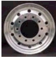
Figure 2.2. Forged Al alloy wheel [12]
