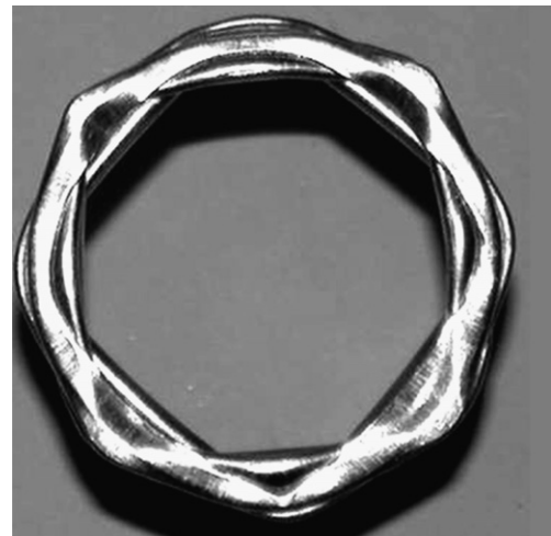
Fig. 6. View of a crushed empty Al tube in diamond mode.
