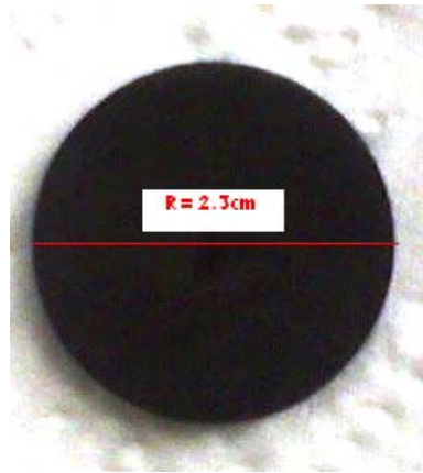
Figure 3.2. Lu doped YBCO target's diameters. The height is 0.26 cm.
